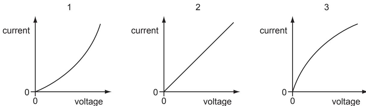
Which graph is for a resistor at constant temperature and which is for a filament lamp?
