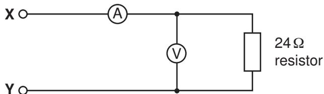
Which pair of readings is obtained when a suitable power supply is connected between X and Y?
