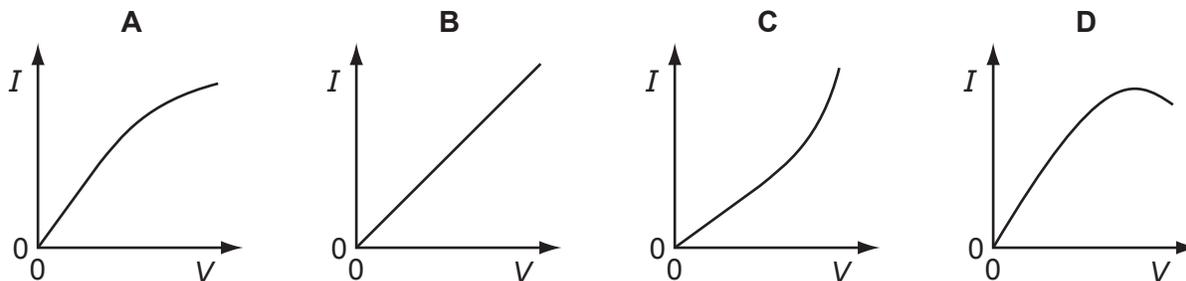
28 The voltage/current graph for a filament lamp is shown.
