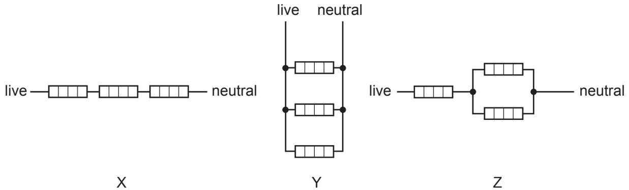
In which arrangement is the current from the supply lowest and in which is it highest?
