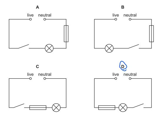
Which diagram shows a lamp wired correctly to the mains supply in a house? 5
