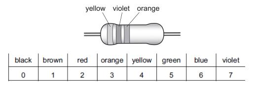
Using the key provided, what is the resistance of the resistor?
